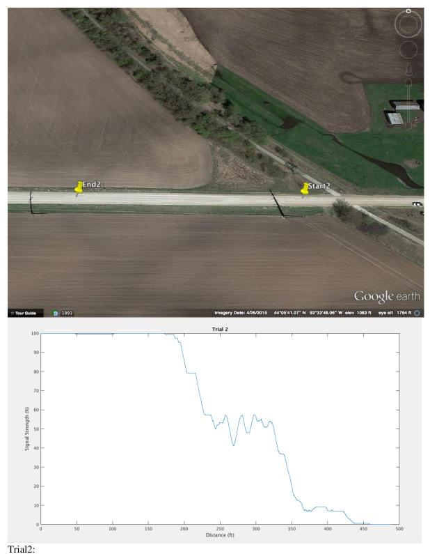
Trial2: (Deg,min,sec) Start: 44°05'38.2"N 92°33'45.2"W End: 44°05'38.2"N 92°33'51.9"W Distance=489ft 149m
